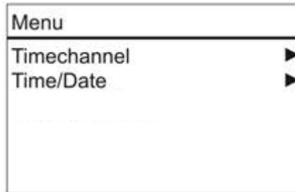
Keys (5), (6), (7) and (8) can be used to navigate through the menu. The On/Off key confirms the adjustments performed. The user accesses a sub-menu by navigating to the required menu using keys (5) and (6) and using key (8) to open it. If the cursor is positioned in the header, key (7) can be used to open the higher-level menu. The Parameter menu is automatically exited after 60 seconds with no input. The values are stored if key (7) is used to exit a sub-menu.
