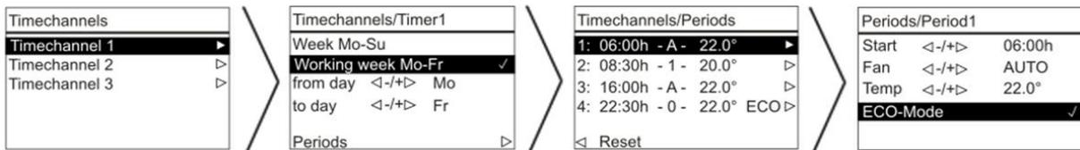
Once the line of the timer channel to be processed has been selected, key (8) is used to call up the next sub-menu. There is an option of selecting an entire week, a working week or any period within a week. A starting time, a setpoint temperature and a fan mode (Off/Auto) can then be prescribed for the 4 different time segments in the following sub-menus and the ECO-Modbus can be activated if necessary.
