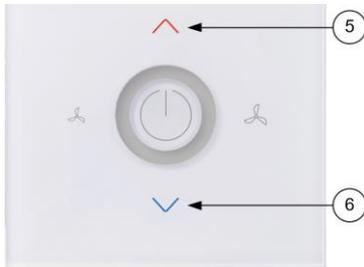
To configure the Modbus interface, please open Modbus settings by pressing 5 and 6 simultaneously for approximately 3 seconds.
