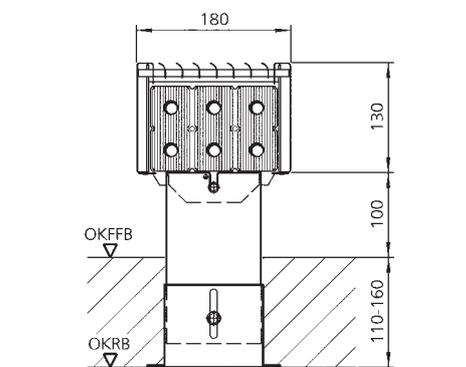
Diag. 7 Section through an unfinished floor unit.
