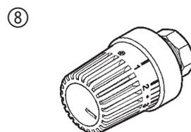
Diag. 2 Thermostatic valve head, type 110210
