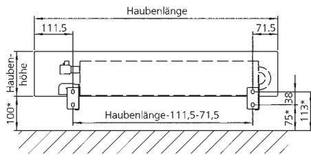
Diag. 8: Bracket spacing - wall-mounted units
