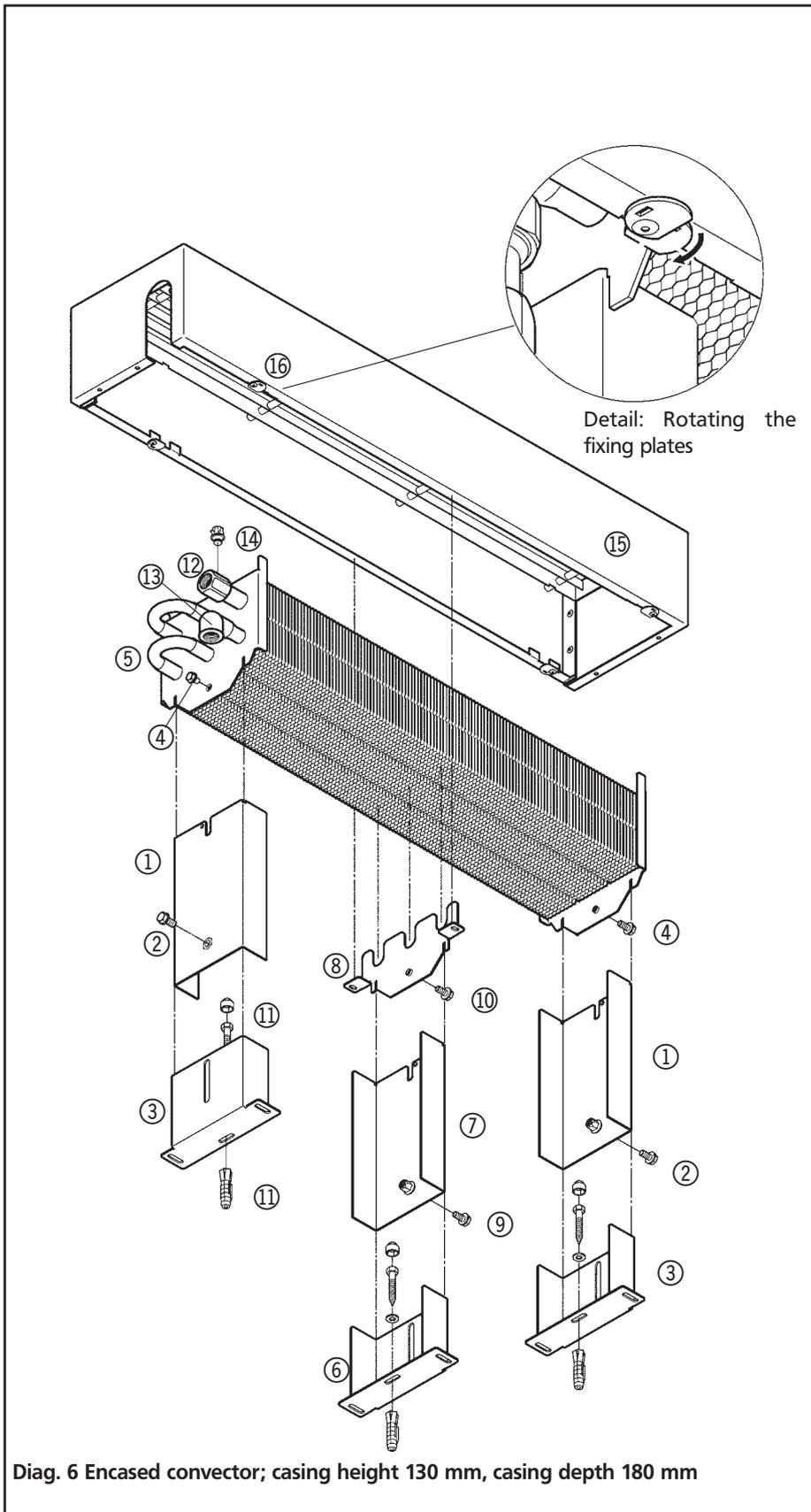
Diag. 6 Encased convector; casing height 130 mm, casing depth 180 mm
