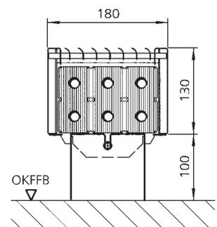
Diag. 5 Section through a finished floor unit.
