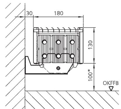
Diag. 10 Section through wall-mounted unit
