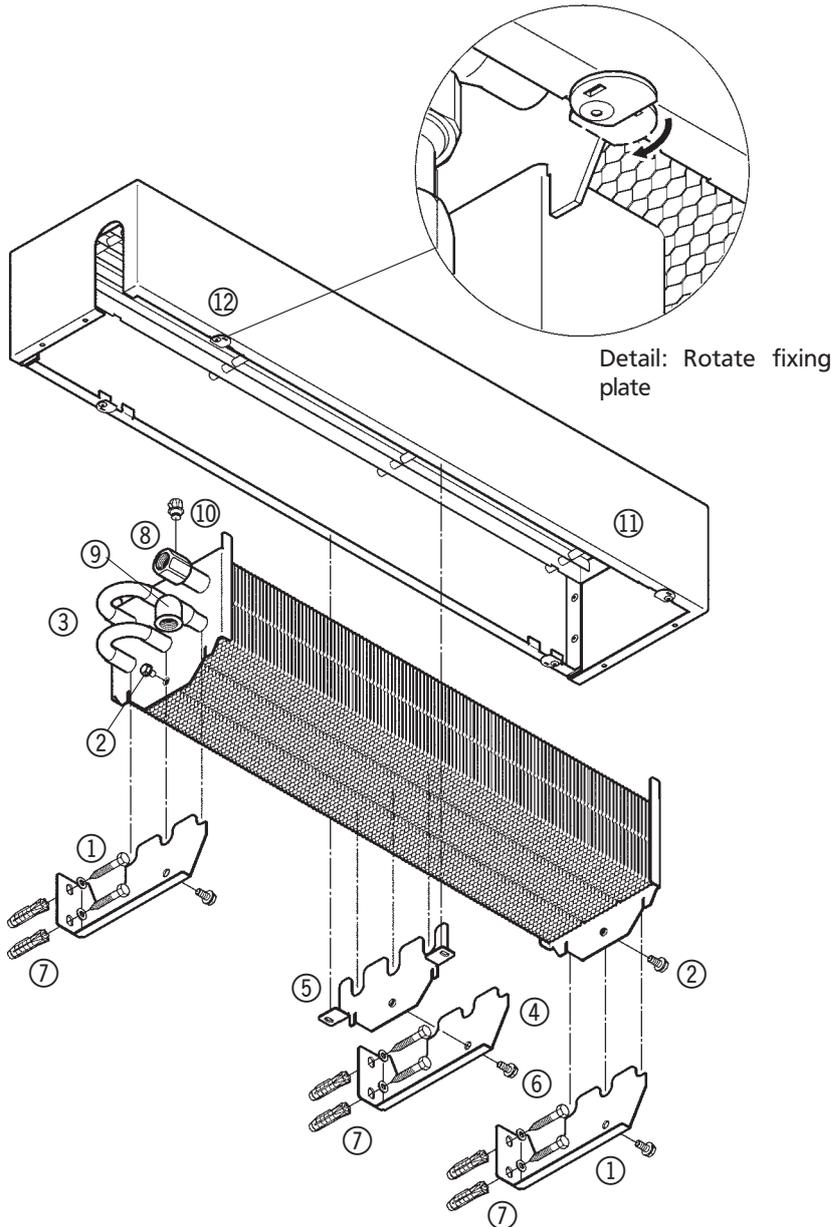
Diag. 9 Encased convector; casing height 130 mm, casing depth 180 mm
