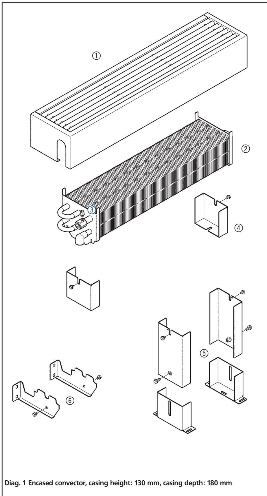
Diag. 1 Encased convector, casing height: 130 mm, casing depth: 180 mm
